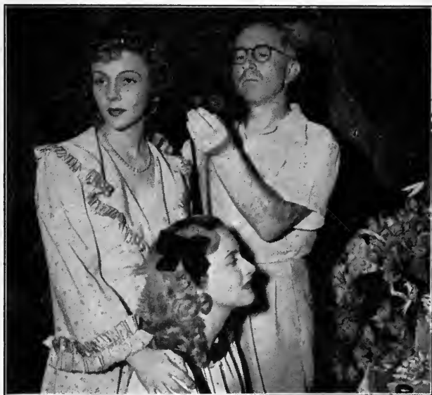
FIG. 3. Showing position of photoelectric cell meter in obtaining key-light; Cinematographer Victor Milner. (Courtesy Paramount Pictures, Inc.)
